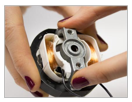
Place the metal axle bridge on the new electro motor.
