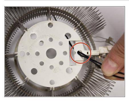
Thread the wire connected to the new electro motor through the right hole in the pastic motor housing.
