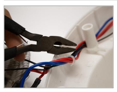
Remove the tie wraps around the wires to allow some space to reach the electro motor.
