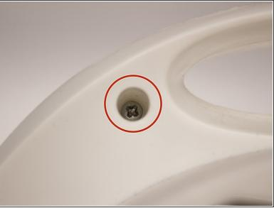
Finally put the two housing halves back together and secure the nine screws.
