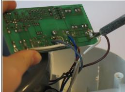
Desolder the two spots connecting the fuse to the PCB. If you have never done this before, use this guide from iFixIt.
