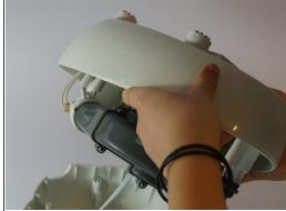
Use a Phillips screwdriver to loosen the screws, then turn the product right side up to get the screws out of the casing.
