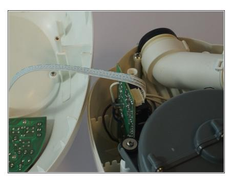
Place the product on its feet and place the upper part of the casing next to the bottom part.
