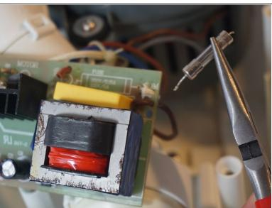
Take out the fuse with some pliers, since it will be hot because of the soldering.
