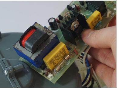
Put in a new fuse and solder it back in place. Now you can reassemble the product.
