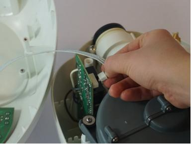
An electronic wire is connecting the two PCB's. Take off the PCB in the lower part of the case by gently pulling the plastic housing, the connection will slowly loosen.
