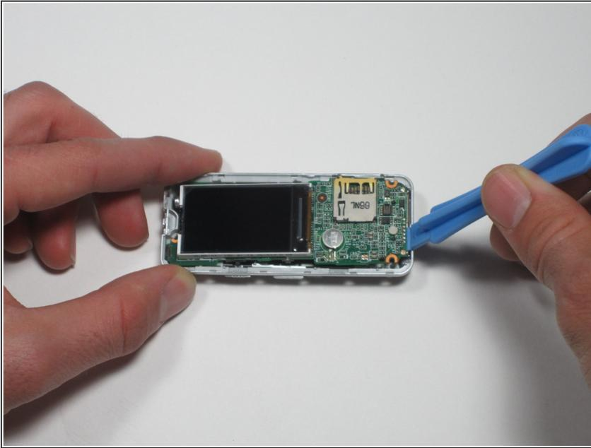
**⚠ CAUTION:** Do not scrape the spudger along the top of the motherboard or you may damage the circuitry.
