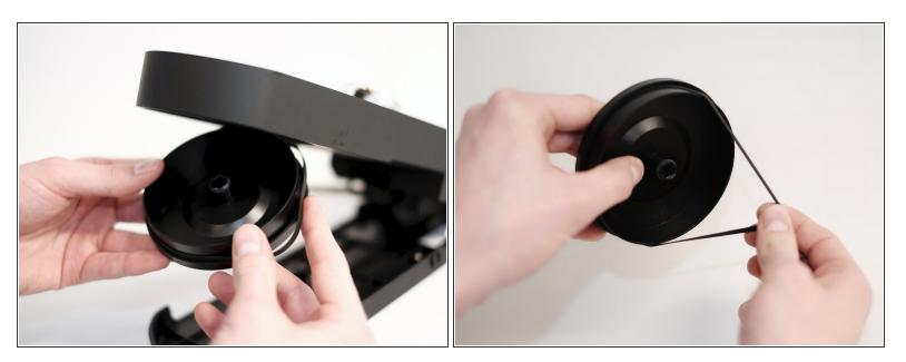
Carefully removed the rubber band from around the motor and extract the turntable from the device.
