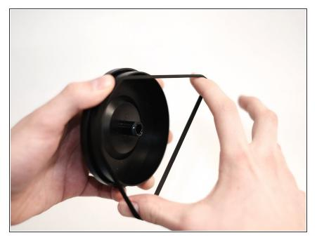
• Remove the damaged belt. Place the new belt around the turntable.
