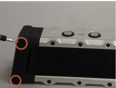
Begin by unscrewing the four 10.72mm corner screws using the Hex 2.0 screwdriver.
