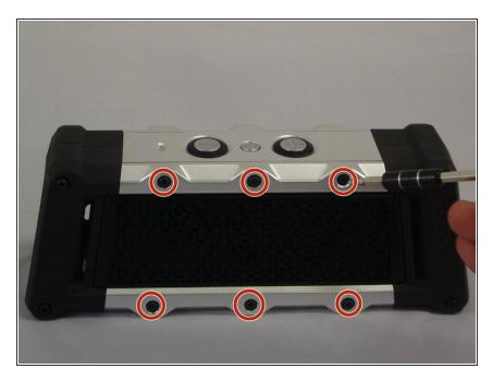
Using the Hex 1.5 screwdriver remove remaining 6-5.79mm screws on the front of the speaker.
