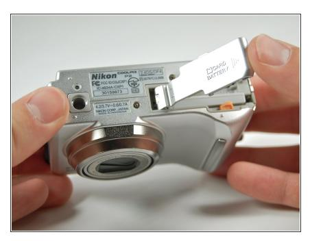
Open battery door by applying pressure to the right.
