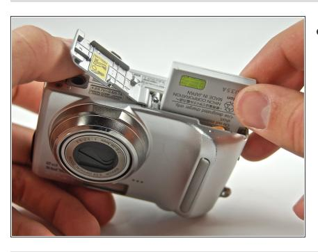
Remove the battery by pulling it out of the slot.
