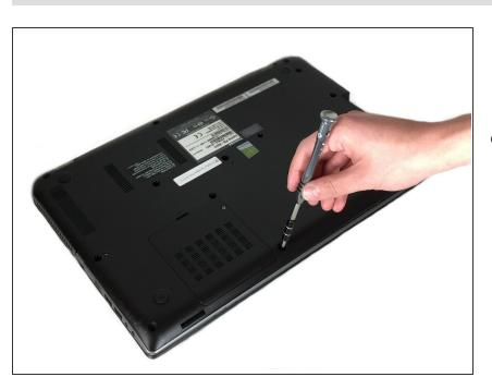
After all rubber plugs are removed, use a Phillip's head screw driver to unscrew all previously covered screws.
