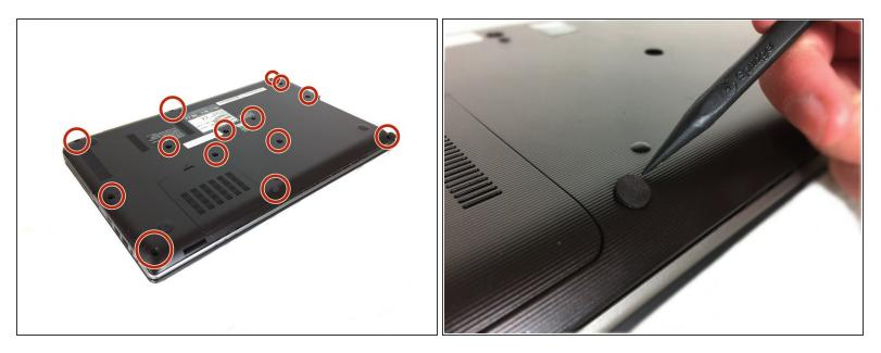
Locate all rubber plugs on the bottom of the laptop. These will need to be removed with a pointed object like the Spudger.
