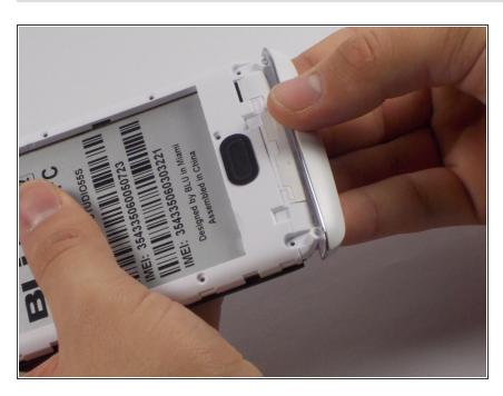
Apply pressure and pop off the bottom aesthetic case, being careful not to break it.
