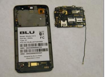
• Use the <u>tweezers</u> to grip the bottom of the motherboard and lift up.
