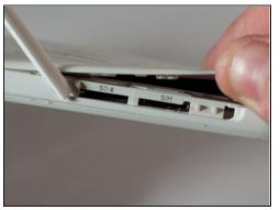
⚠ Before you proceed, discharge your device battery below 25%. A charged lithium-ion battery can catch fire and/or explode if accidentally punctured.
