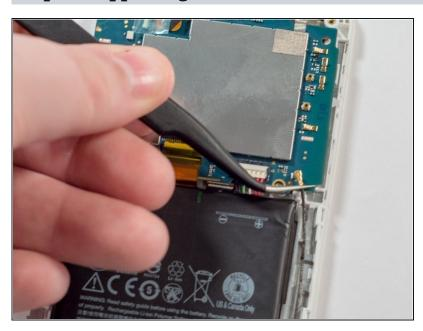
Using the <u>tweezers</u>, remove the antenna connection. Grab the connector by the base and pull towards the head of the connector.
