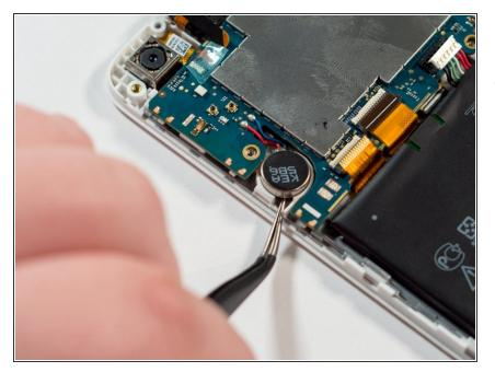
Using the tweezers or another small pointed tool, place the tip under the edge of the round disk-like component on the left side of the device. Apply a small amount of pressure to the edge of the component to dislodge it.
