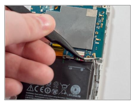
Using the tweezers, remove the antenna connection. Grab the connector by the base and pull towards the head of the connector.
