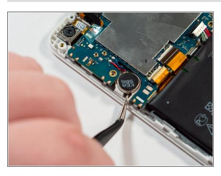
Using the tweezers or another small pointed tool, place the tip under the edge of the round disk-like component on the left side of the device. Apply a small amount of pressure to the edge of the component to dislodge it.
