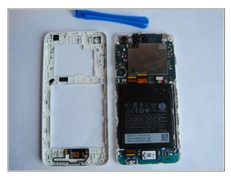
Continue working your way around the seam between the two parts and eventually you will be able to separate the entirety of the backplate revealing the internals of the device.
