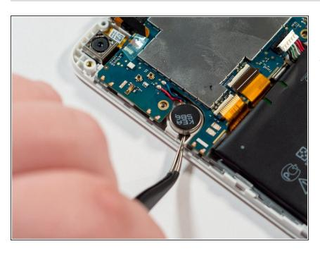
Using the tweezers or another small pointed tool, place the tip under the edge of the round disk-like component on the left side of the device. Apply a small amount of pressure to the edge of the component to dislodge it.
