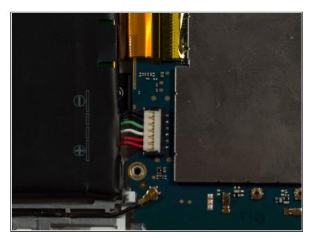
After prying the battery free from the device the connector can be removed by pulling directly up away from the device.
