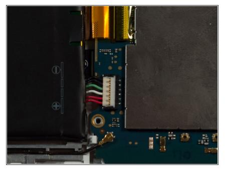
After prying the battery free from the device the connector can be removed by pulling directly up away from the device.
