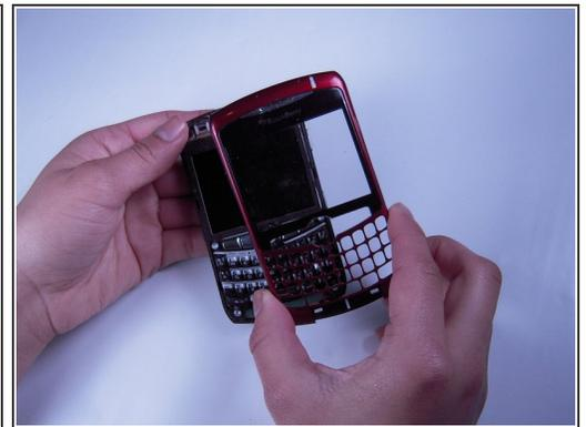
⚠ Be careful not to damage the front cover's plastic clips while trying to separate it from the phone.
