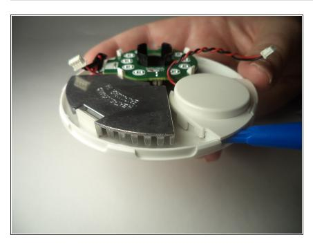
Insert plastic opening tool below the plastic speaker cover on the inside of the removed front panel of the device.
