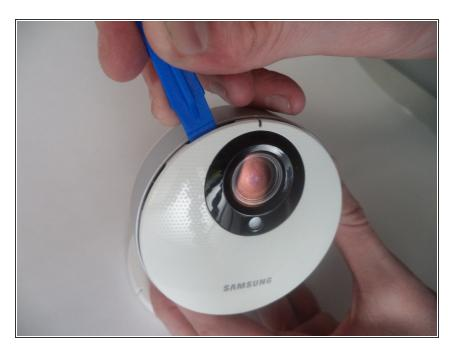
Locate a small opening around the front panel of the camera.
