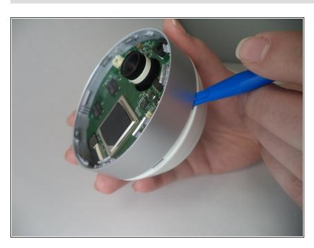
Apply pressure with the plastic opening tool to various areas of the gray plastic band to pry it from the white plastic back of the case.
