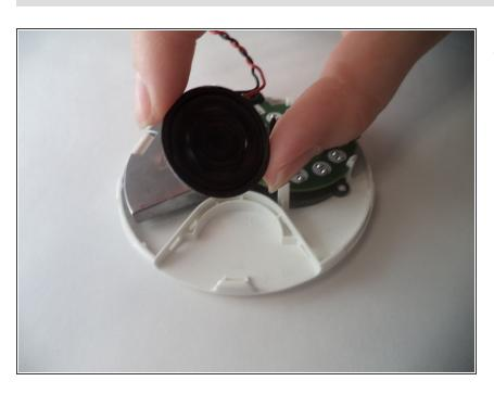
Pull out the speaker which is now loosely resting in its plastic housing.
