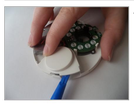
Push the two tabs holding the speaker cover on, while prying it up.
