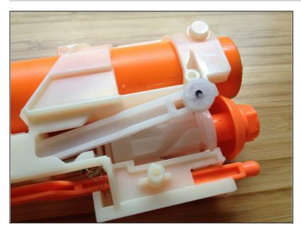
(i) Remove the piece holding the barrel reloading piston.
