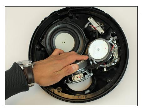
Pull out the speaker, and if necessary follow these steps to replace the other identical speaker.
