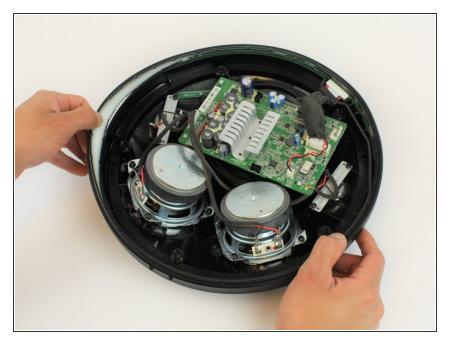
Pull the silicone button band off of the outer edge of the speaker.
