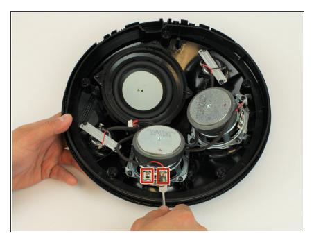
Using the metal spudger, gently pry off the two red and black connectors.
