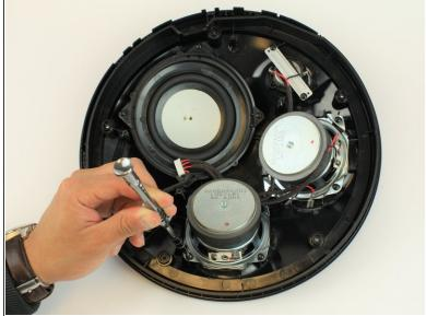
Remove the four 14.3 mm T10 Torx screws.
