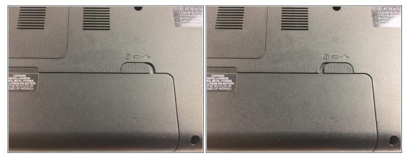
On the right side of the battery there will be a locking switch. Slide the switch into the unlocked position.
