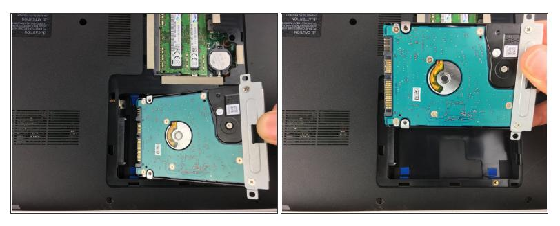
• Then using the tab located on top of the hard-drive pull up towards you and then pull to the left to disconnect the hard-drive. Now you are ready to replace your hard-drive.
