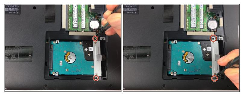
Remove the two 7 mm screws holding the hard-drive in place with a P1 driver
