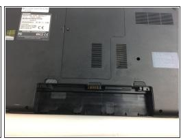
Using your left hand, move the switch on the left side of the battery towards the center of the laptop while simultaneously prying up on the center of the battery with a spudger. The battery will flip out and can be removed.
