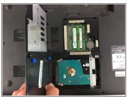
Remove the 7mm screw near the center of the back of the laptop with a P1 screwdriver and pry off the access panel with a nylon spudger.
