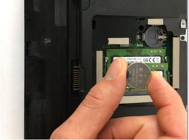
Then using a spudger, try to get under the battery and the battery will pop out of place. You are now ready to replace the CMOS battery.
