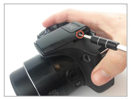
Remove the two screws (5-6mm) on the left and right side of the shutter panel with a Phillips PH000 screwdriver.
