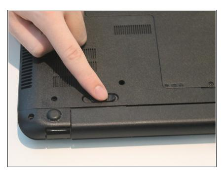
Move the left switch to the right, covering the battery symbol, and hold.
