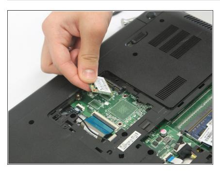
Slide the wireless card to the left to remove it from the socket.
