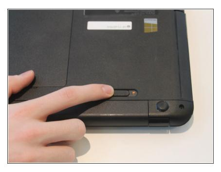
Move the right switch to the left so that the orange unlock symbol is showing.
