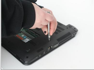
Remove the fourteen Phillips PM2.5×6.0 screws, and place them in a separate container.
