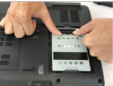
Push the hard drive out of its housing as shown.
