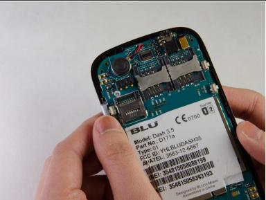
Remove volume and lock buttons by lifting them gently from the casing.
