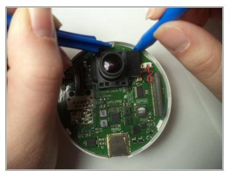
• Press each tab while using a plastic opening tool to pry the motherboard up in the location near the tab.
