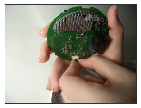
Unplug the final group of wires from the bottom of the second circuit board.
