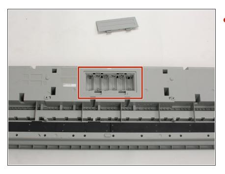
Load six new D-size batteries into battery compartment ensuring the positive (+) and negative (-) ends up with illustration inside of compartment.
