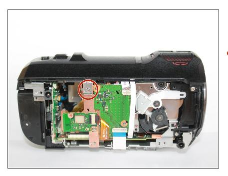
Unscrew indicated screw on the inside of the left side of the camcorder.
