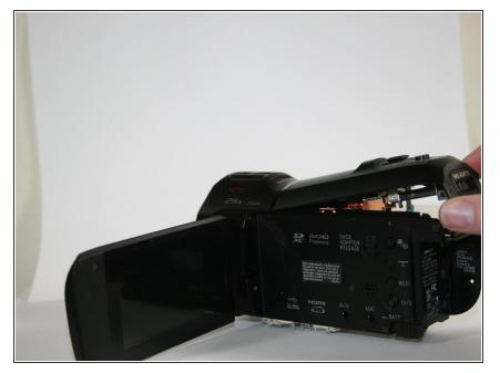
Remove the top cover of the camcorder by lightly lifting up on the back end of the top and tugging away from the lens (don't be afraid to use force).
