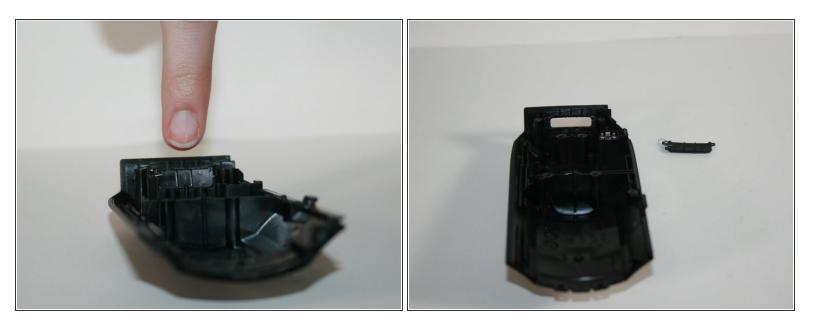
• Remove the shoe adapter by simply pulling it out of its place.
