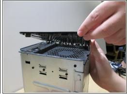
With case removed push tabs on back cover to remove the back cover. You can do this with your fingers or a tool such as a spudger.
