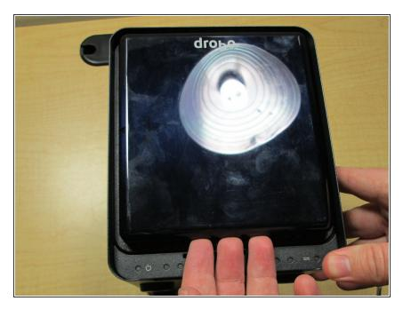
To start getting the case off remove the front panel so it's out of the way.
