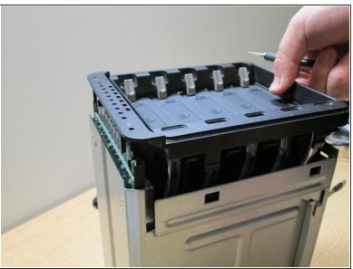
• Then do the same to the other side, pushing the pins down. Then slide the hard drive docks out.
