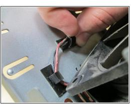
Next remove the fan by placing your screwdriver through the holes so that you can push out the small rivets. Then unclasp the wires so that you can finally remove the fan.
