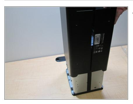
To remove the case, place the Drobo on its back and slide the case off.
