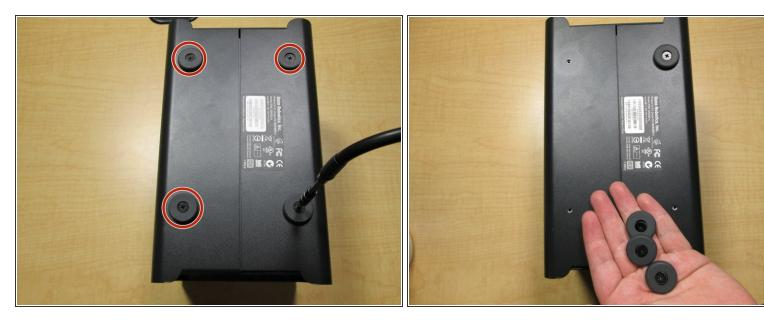
Next remove the screws from the feet of the case with a phillips head screwdriver.
