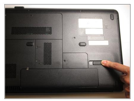
Flip the computer so that the backside is facing you. Locate the button shown.
