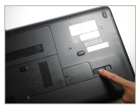
Push this button to the left and it will release the battery.
