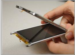
Marning: If you are too rough with the screwdriver, you can permanently damage the display.
