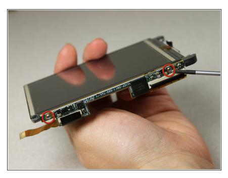
Unscrew the 2 Philips #00 screws from the bottom edge of the screen component.
