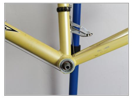
The Bottom Bracket is located at the bottom of the frame, directly underneath the saddle.
