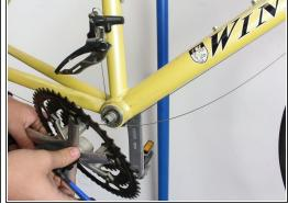
Once the movable piece is tightened firmly inside the hole, turn the tool clockwise. This will pull the crank arm away from the bike and remove it completely.
