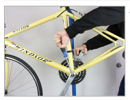
To remove the crank arm, place a proper fitting Allen wrench into the slot at the center of the crank arm as shown. Turn the wrench counterclockwise to loosen the bolt that keeps the crank arm on the bike until it spins easily. Hold the other crank arm in place to ensure that the bolt loosens instead of spinning the crank arm.
