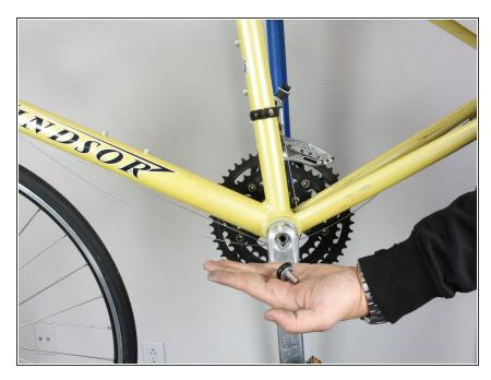
Remove the bolt from the crank arm.
