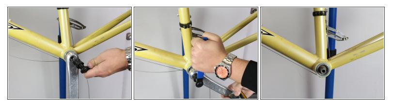
Repeat steps 6-7 with the remaining crank arm. Both arms have been successfully removed.
