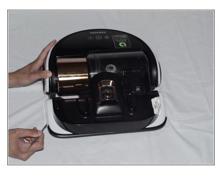
Use a tool to pry this sensor away from its holdings. This may require a little bit of extra force.
