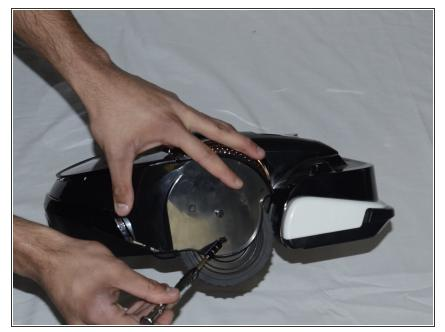
For the wheel you want to remove, there is a small square opening on outer black protective layer still around the wheel. Locate the screw that is inside the whole. Remove this screw.
