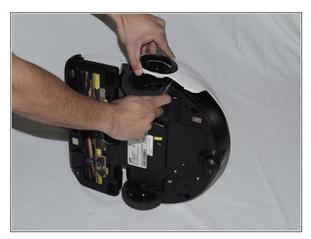
Next, pry and remove the white casing that runs around the back round part of the bot.
