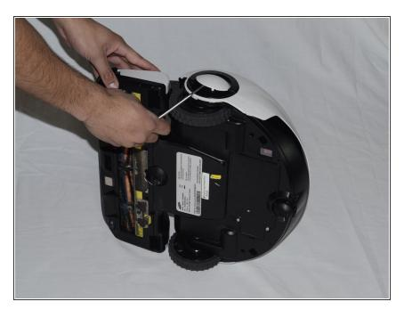
Flip the bot onto its side with the wheel you want to remove on top.
