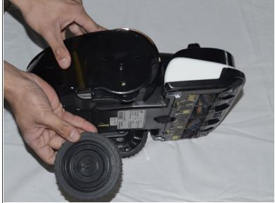
Pry the black protective layer away from the wheel, and pull the wheel out.
