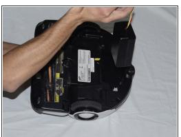
• Push this tab into the white box, and pull the wires up. This releases the wire from the white box, allowing you to fully remove the battery.
