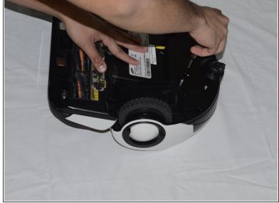
Unscrew each of the two screws and remove the lid to expose the battery.
