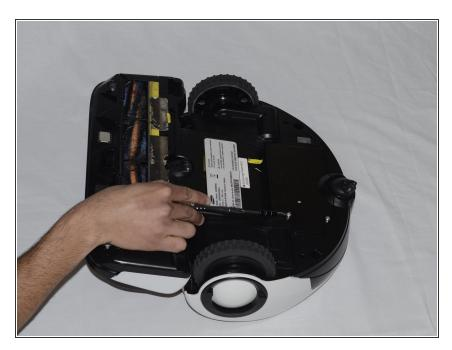
On the bottom of the bot, locate the battery lid along the curved edge of the bot.
