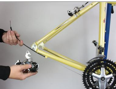
Using a hex key wrench, unscrew the bolt that fastens the derailleur to the bike frame. The
