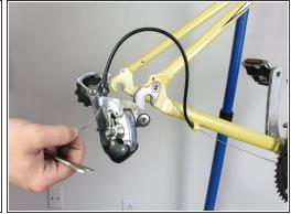
Using a pair of wire cutters, locate the end of the derailleur cable. Cut the wire just below the cap, cutting off the metal end piece.
