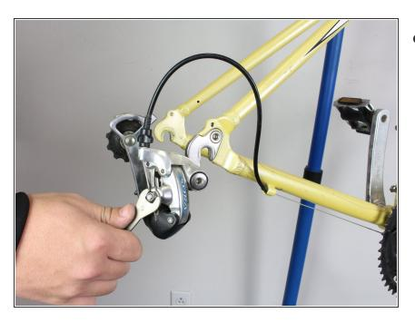
Loosen the hex nut, as shown, on the side of the derailleur. This bolt plays a key role in securing the derailleur cable which we will need to cut in step two.
