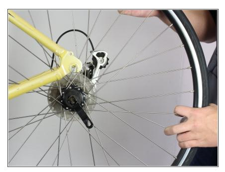
When the quick release is opened, the wheel is ready to remove.
