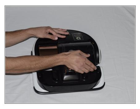
For stability, place one hand on the curved back edge of the bot, and place the other on this pull handle.
