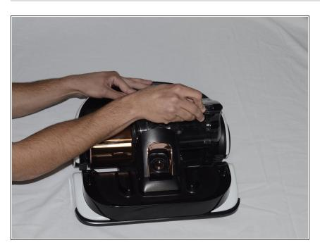
Pull the handle up and towards the back of the bot, so the dust bin begins to rotate.
