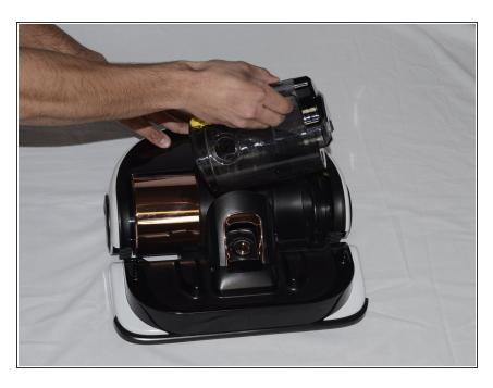
Keep pulling until the dust pin fully releases itself from the bot.
