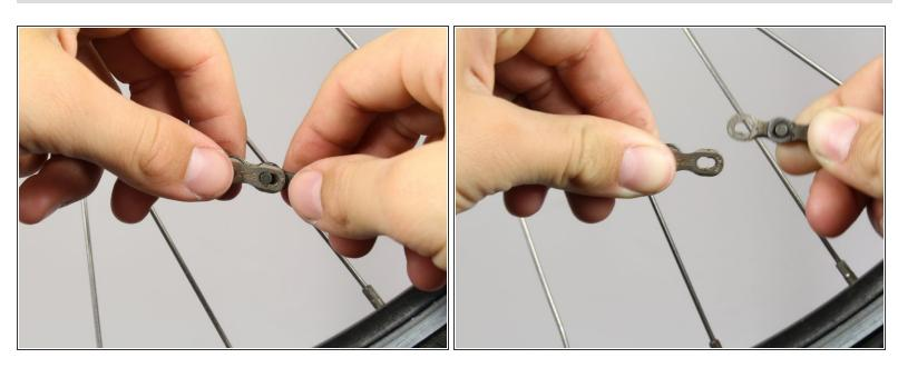
• To separate the Master Link, hold the left side of the link in your left hand and the link to the right in your right hand. Push the two links together to enable the release. Pull the links apart, one hand moving towards yourself and the other away from you. This will separate the links of the chain.
