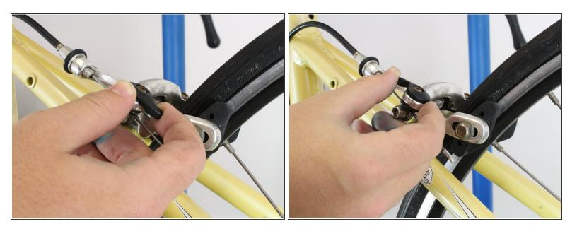
Open the sidepull brakes by fully rotating the title lever on the brake upwards.
