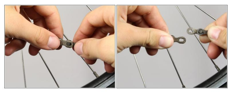
• To separate the Master Link, hold the left side of the link in your left hand and the link to the right in your right hand. Push the two links together to enable the release. Pull the links apart, one hand moving towards yourself and the other away from you. This will separate the links of the chain.
