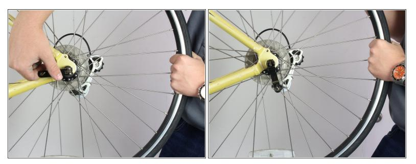
To loosen the wheel, simply pull out the lever, away from the frame and loosen up.
