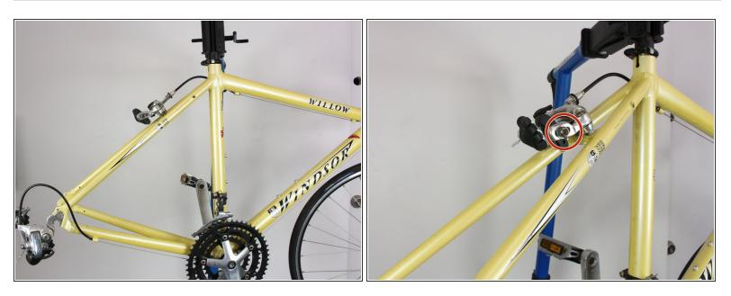
• The hex bolt is what fastens each brake pad to the caliper. We will need to remove these to replace each pad.
