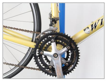
• The chain connects the crank arm to the gear cluster on the back wheel.
