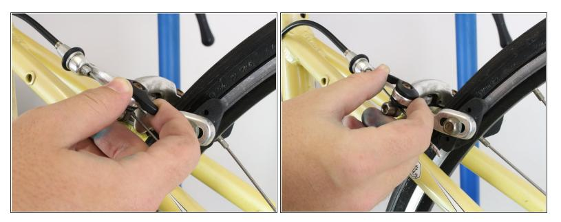
• Open the sidepull brakes by fully rotating the title lever on the brake upwards.
