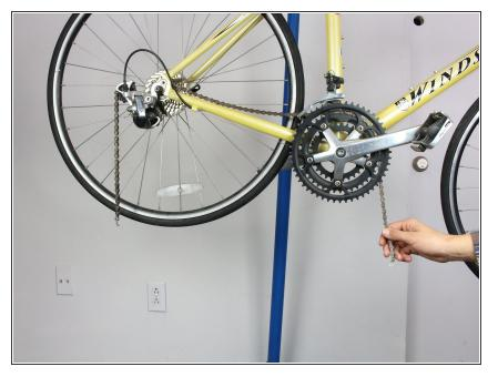
Once you have separated the links of the chain, pull down on the right side of the chain as shown. Pull until the chain has been fully removed from the gears. Place the chain on a paper towel or cloth to prevent getting grease anywhere.
