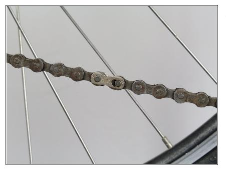
On the chain, locate the master link. It is a lighter gray than the other links of the chain. This is how you can break the chain for easier removal.
