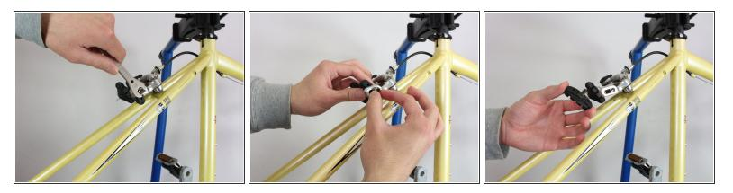
• Using an open end 10mm wrench, unscrew the hex nut from the caliper. After the nut is loosened you can use your fingers to finish the job. Repeat the same process on the other side for removal of the second brake pad.
