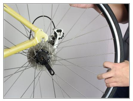
• When the quick release is opened, the wheel is ready to remove.
