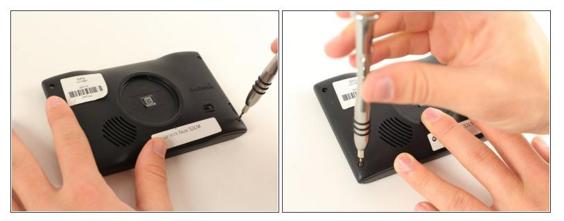
Place the device face-down, with the screen facing the surface. There are 8.7mm screws located in each of the back 4 corners of the device. Using a T5 Torx screw bit, unscrew all four screws and leave them aside.
