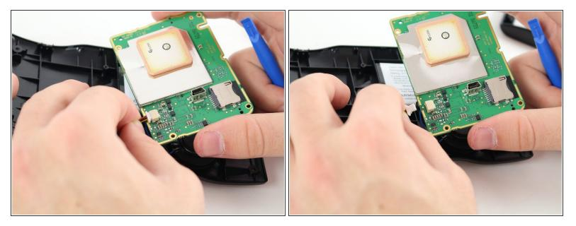
Gently unplug the wire connecting the battery to the small socket on the back of the motherboard.
