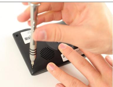
Place the device face-down, with the screen facing the surface. There are 8.7mm screws located
