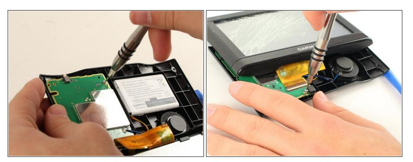
Using the T5 Torx screwdriver, unscrew the two 5.6mm screws at the top right and bottom right corners of the motherboard.
