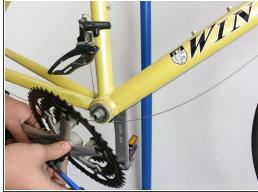
Once the movable piece is tightened firmly inside the hole, turn the tool clockwise. This will pull the crank arm away from the bike and remove it completely.
