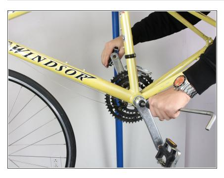
Once the bolt spins easily, keep the Allen wrench in the bolt slot and turn the crank arms to speed up the removal process.
