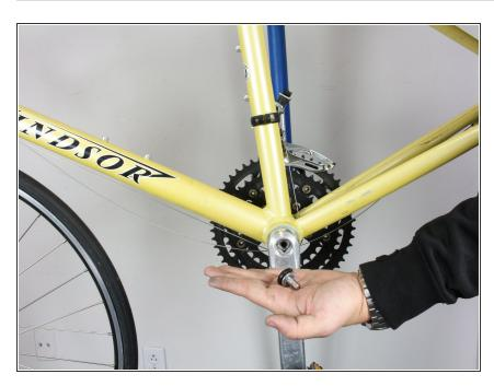
Remove the bolt from the crank arm.
