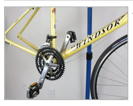
The crank arms can be located between the front and rear tire, directly below the seat.
