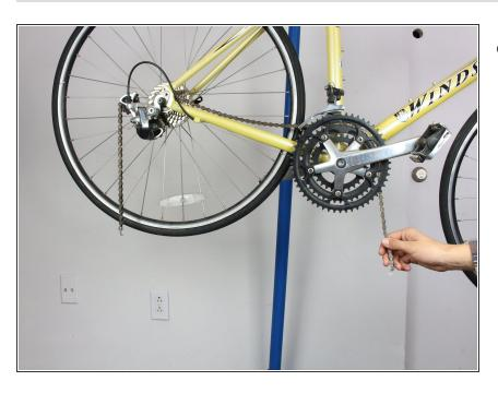
Once you have separated the links of the chain, pull down on the right side of the chain as shown. Pull until the chain has been fully removed from the gears. Place the chain on a paper towel or cloth to prevent getting grease anywhere.
