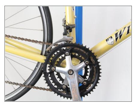
The chain connects the crank arm to the gear cluster on the back wheel.
