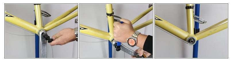
• Repeat steps 6-7 with the remaining crank arm. Both arms have been successfully removed.
