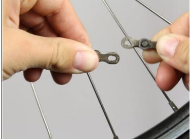
• To separate the Master Link, hold the left side of the link in your left hand and the link to the right in your right hand. Push the two links together to enable the release. Pull the links apart, one hand moving towards yourself and the other away from you. This will separate the links of the chain.
