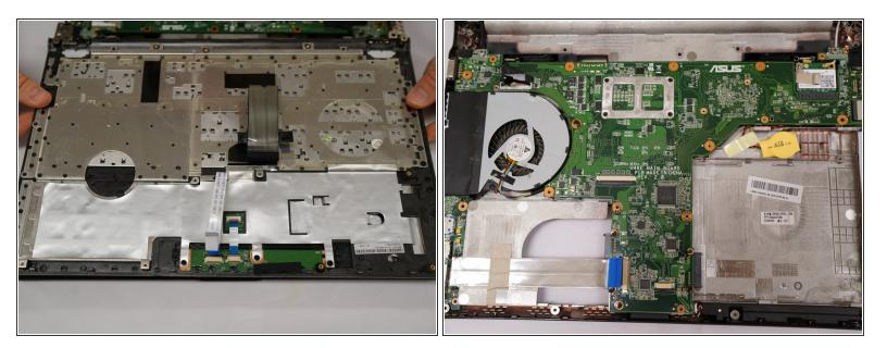
• Remove the keyboard from the computer to reveal the motherboard.
