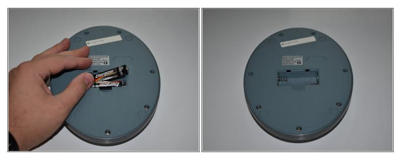
• Use the plastic tab to pry the battery cover off to get the batteries up and out of the device.
