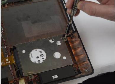
• Using the screwdriver with the JO bit, remove the two Phillips 4 mm head size 5 mm long screws from the Hard Drive.
