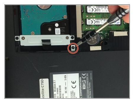
Remove the 3mm screw located under the back access panel nearest the optical drive with a P1 driver.
