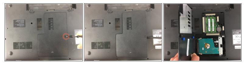
• Remove the 7mm screw near the center of the back of the laptop with a P1 screwdriver and pry off the access panel with a nylon spudger.
