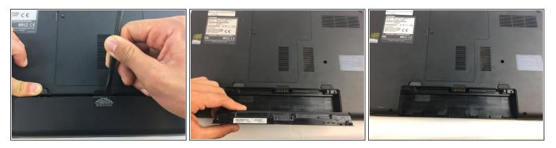
• Using your left hand, move the switch on the left side of the battery towards the center of the laptop while simultaneously prying up on the center of the battery with a spudger. The battery will flip out and can be removed.
