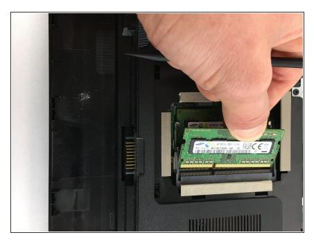
• Gently pull the RAM module out of the laptop and repeat for the second module.
