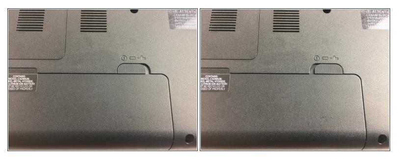
On the right side of the battery there will be a locking switch. Slide the switch into the unlocked position.
