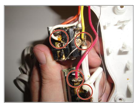
• Verify wires are connected to each switch and are in good condition
