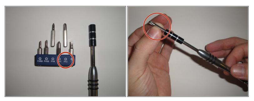
• Remove the bit from the screwdriver and insert the Phillips PH2 bit
