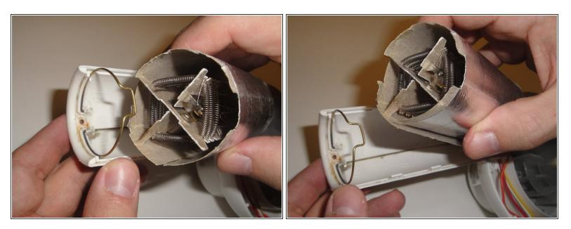
• Pull up and remove the heating element assembly
