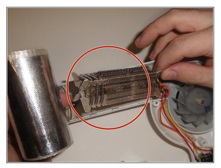
• Remove the outer sleeve and replace the heating element
