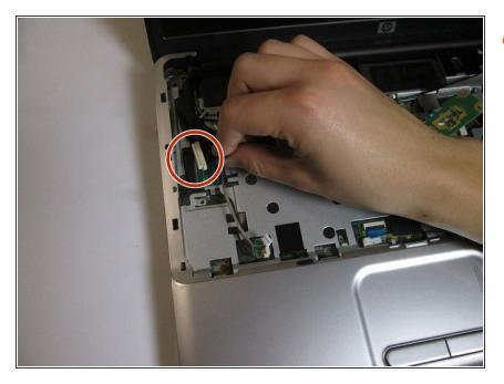
Remove the covered cable ribbon that is located at the left side of the computer.
