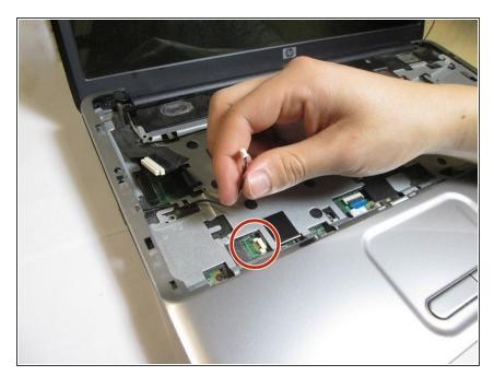
• Gently pull the smaller wire from its clip. Please do not pull the wire by holding the wire itself. Use the plastic cover to pull.
