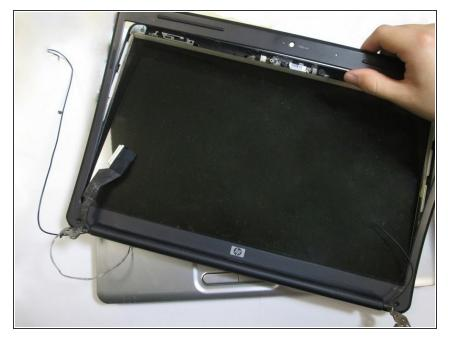
• Firmly pry the front screen cover off. Slide the prying tool around the front screen. Please be careful not to destroy the clip. It will destroy the entire screen.
