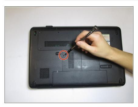
• Lay the computer so that the backside is facing you and locate the screw in the picture.
