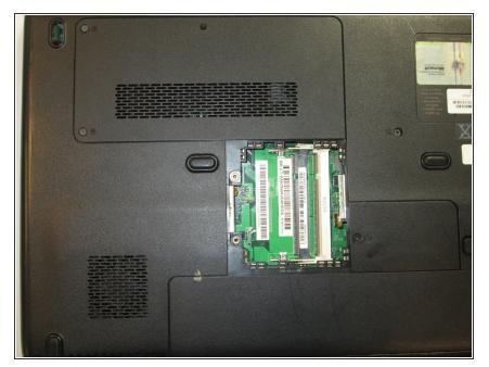
Remove each one of the rams so that the computer looks like this. You can do so be squeezing tabs on each side of the ram.
