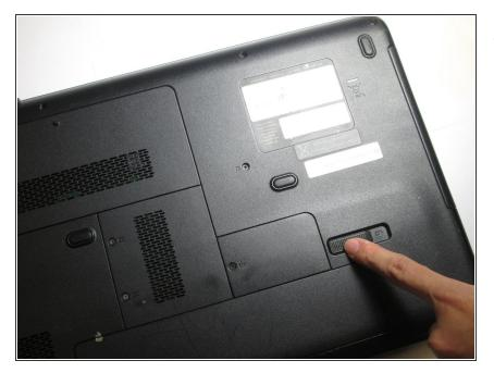
Push this slide over in order to remove the battery. This is safe when working with your computers memory.
