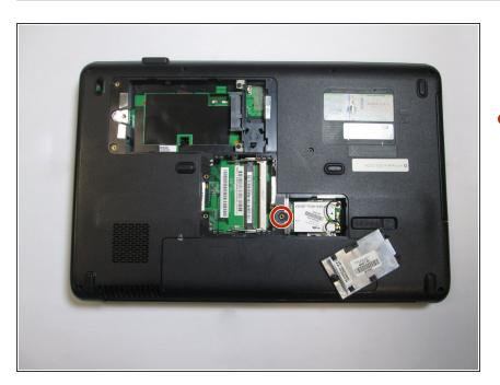
Using a screwdriver, remove the 3 mm screws holding together the plate found in the directly right of the central plate.
