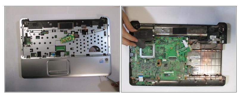
• Use a spudger to remove the remaining keyboard plate on the front of the laptop body.
